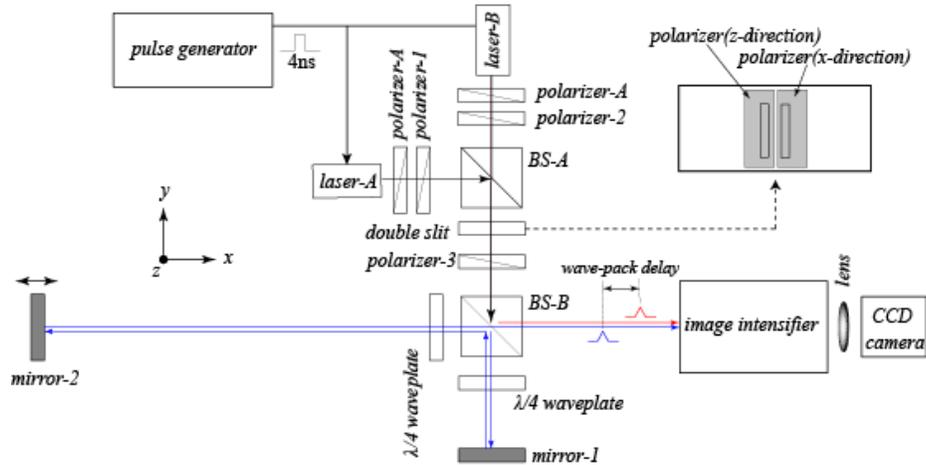
Fig. 5 Apparatus to observe the fourth-order interference using short (red) and long (blue) optical paths. A wave packet of approximately 4 ns is emitted from the independent lasers. The polarizing plate is arranged so that each light wave passes through only one of the double slits. The wave packets are divided by the polarizing beam splitter BS-B into a short optical path and a long optical path, and they enter the image intensifier.
