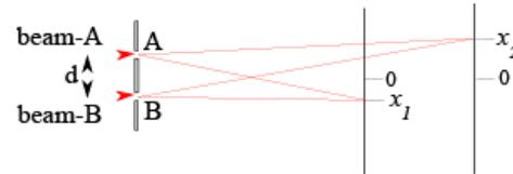
Fig. 4 Optical system to observe the fourth-order interference obtained in two spatially separated regions
