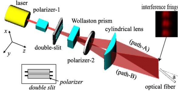
Fig. 1. Modified double-slit interferometer. The polarizing plates in the x- and y-directions are attached to each slit of the double slit. The optical fiber is on the yz-plane and inclined at approximately  $6^\circ$  (denoted by "a") from the z-axis.
