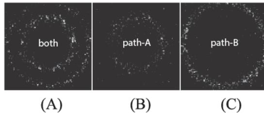
Fig. 2. (A) CCD image of the light wave emitted from the fiber when path A and path B are opened; (B) and (C) images when only either path A or path B is opened.
